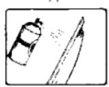
SPRAY or brush on a mold release to both the Quick-Release and your mold. Add extra coats for the bowl molds.
